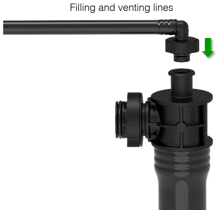
Fig. 16: Central placement of the filling and venting line above the connection contour of the venting valve
